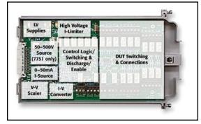
Three source/switch plug-in modules provide the Model 2790 with programmable high voltage and low current sources, connection switching, and signal conditioning circuitry.
