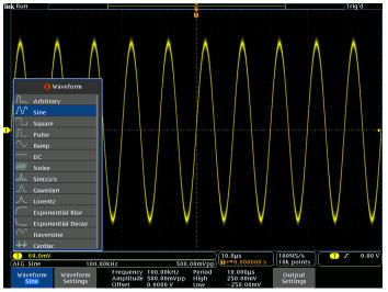
Waveform type selection in the integrated AFG.
