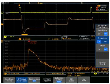
The orange waveform in the Time Domain view is the frequency vs. time trace derived from the spectrum analyzer input signal. Notice that Spectrum Time is positioned during a transition from the highest frequency to the lowest frequency, so the energy is spread across a number of frequencies. With the frequency vs. time trace, you can easily see the different frequency hops, simplifying characterization of how the device switches between frequencies.
