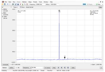
The wide-bandwidth, high dynamic range options (B85HD, B125HD, and B16xHD) offer unmatched real time spectrum analysis dynamic range. Two 16-bit, 200 MS/sec digitizers are interleaved, resulting in 400 MS/sec acquisitions with a typical spurious free dynamic range of -80 dBc, up to 10 dB better than other commercially available instruments. Here, a signal at 3 GHz is measured at -13.71 dBm, with the largest spurious signal from the digitizer -87.89 dB below the carrier.
