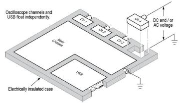
Isolated-channel technology is specified to 1000 V<sub>RMS</sub> maximum float voltage
