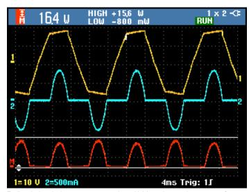
Easily calculate the instantaneous power by multiplying voltage and current waveforms
