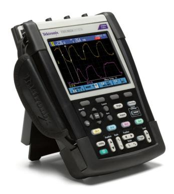
With two isolated channels and up to seven hours of battery life, the lightweight THS3000 Handheld Oscilloscope Series enables you to safely make floating or differential measurements on your bench or in the field. Now you can tackle tough environments with the performance you expect from Tektronix - safely and affordably.
